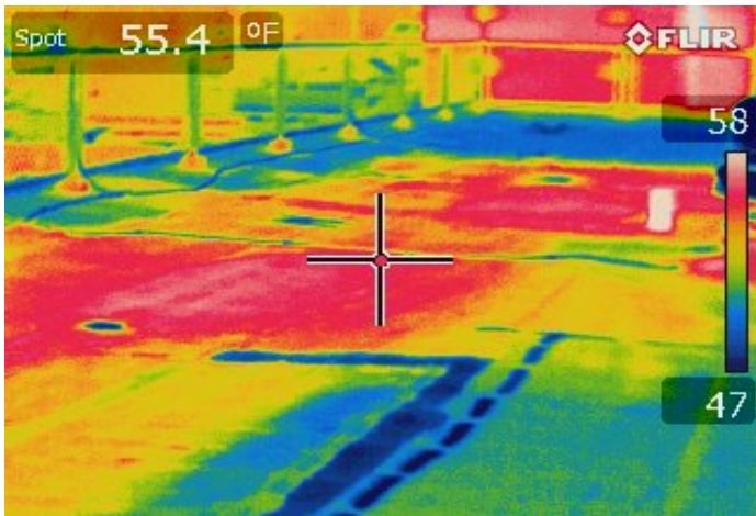
Area(s) where red are being shown were noted as being wet-to-saturated – note temperature of 55.4F° v 50.9F° for Blue, or dry area are(s) as noted
